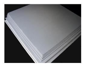
The millboard maintains its strength and thermal stability throughout a wide temperature range up to 2300°F, has a close thickness and dimensional tolerances, and is easily die-cut. These features make it an excellent choice for many gasketing applications in a wide range of industries and applications. The high density and compressive resistance make it an ideal product for refractory backup insulation, as compared to lower density vacuum formed boards or more compressible paper products.
